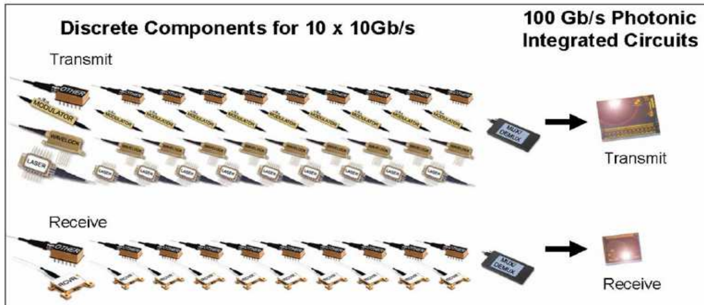
Figure 1: Large-scale Photonic Integrated Circuits enable monolithic integration of over 60 discrete optical components.
